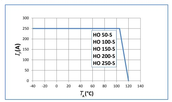
Important notice: whatever the usage and/or application, the transducer primary bar temperature shall not go above the maximum rating of 120 °C as stated in page 2 of this datasheet.
